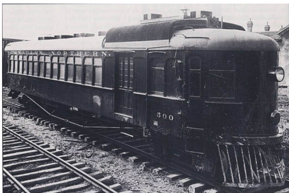
A gas-electric car, similar (or maybe the same), as the one used on the Lochside line.
